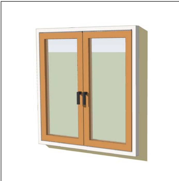
HANDLES DOWN BOTH SASH ARE LOCKED AND SECURE
