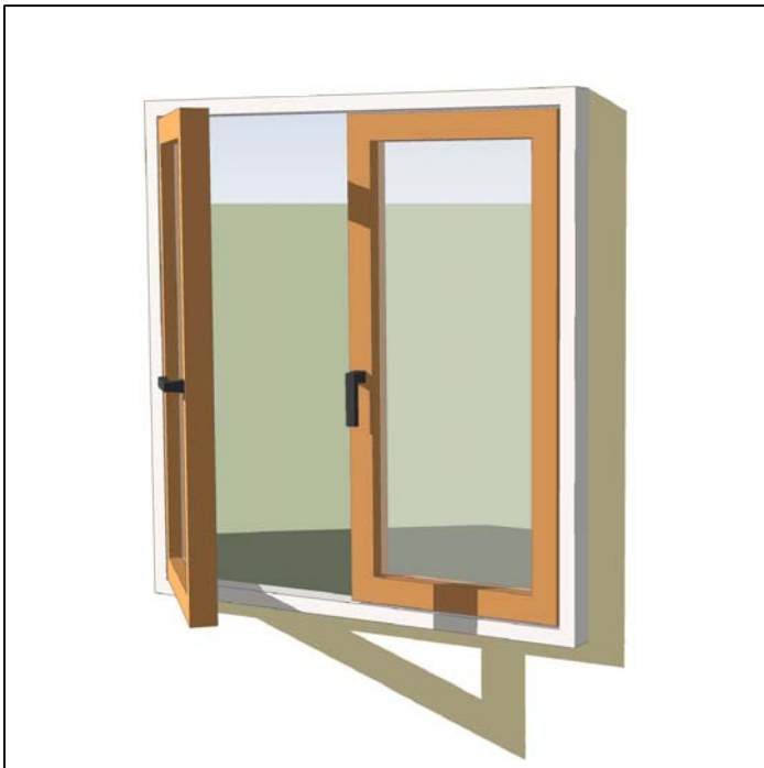
ACTIVE HANDLE SIDE PRIMARY SASH CAN BE OPENED, TO ALLOW SECONDARY SASH TO OPERATE
