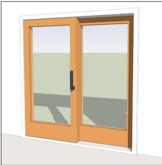
HANDLE UP DOOR PANEL IS LOWERED INTO A LOCKED AND SEALED POSITION
