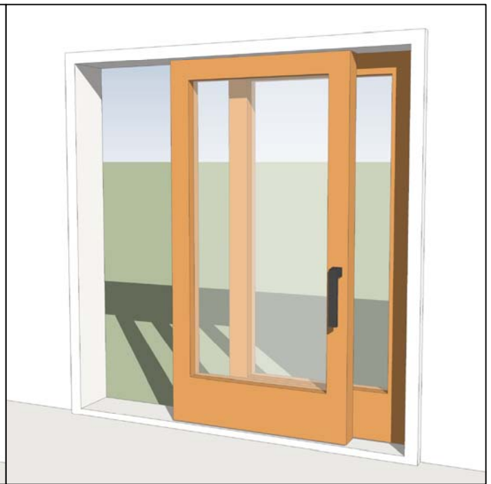
HANDLE DOWN DOOR PANEL IS LIFTED ONTO ROLLERS AND SLIDES EASILY
